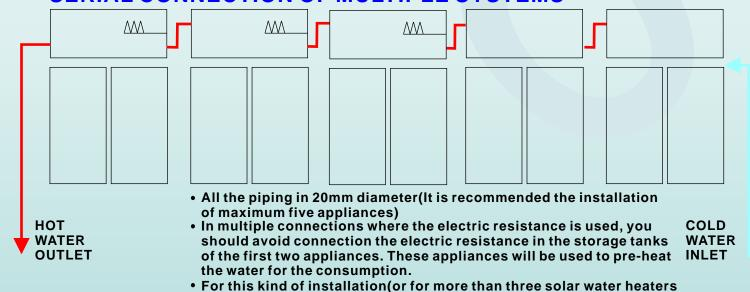
connected in a row) you have to make a special request for inlet-out lets pipes on the storage tank. We recommend you to use a maximum of
